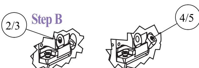
Hand tighten wedge (2) using screw (3).
