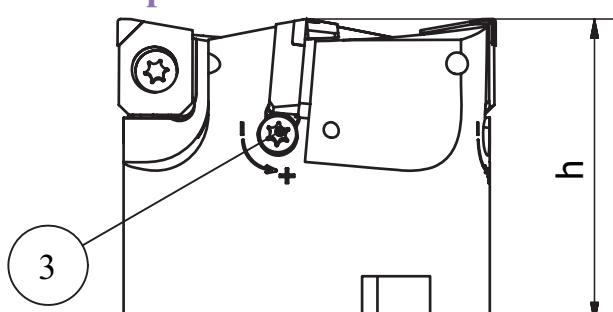
Preset to nominal size  $h$  using screw (3) (axial correction 0.05 max.).
