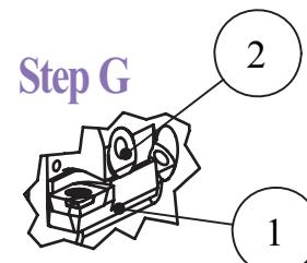
Clamp cartridge (1), using wedge (2),
