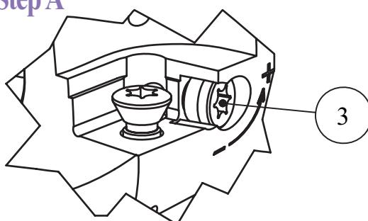
Tighten adjusting screw (3) (left)
