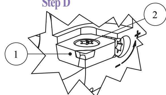
Finally tighten insert (1)
