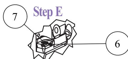
Install insert (6) and fasten using Torx screw (7)
