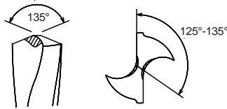
Heavy Duty Notched Point Pointe Entaille à grand rendement Eingekehrte Spitze Schwereinsatz Punta ranurada para uso intensivo Усиленная вершина Notched Point
